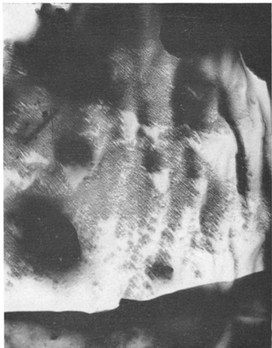
Figure 4 66 Nylon fractograph. Draw ratio \times 5.8(\times 18030) .
