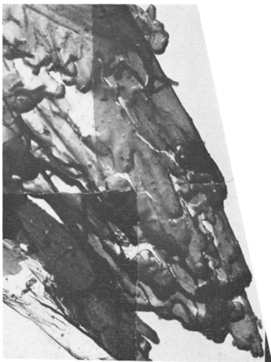
Figure 1 66 Nylon fractograph. Draw ratio \times 5.8 ( \times 9900 ).
